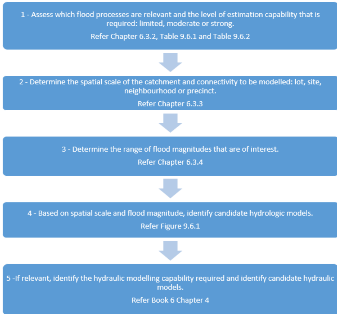
Figure 9.6.2. Stepwise Flowchart for Selecting an Urban Stormwater Model
