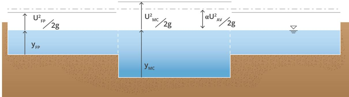
Figure 6.2.9. Variation of the total energy grade line across the compound channel section assuming a horizontal water surface.
