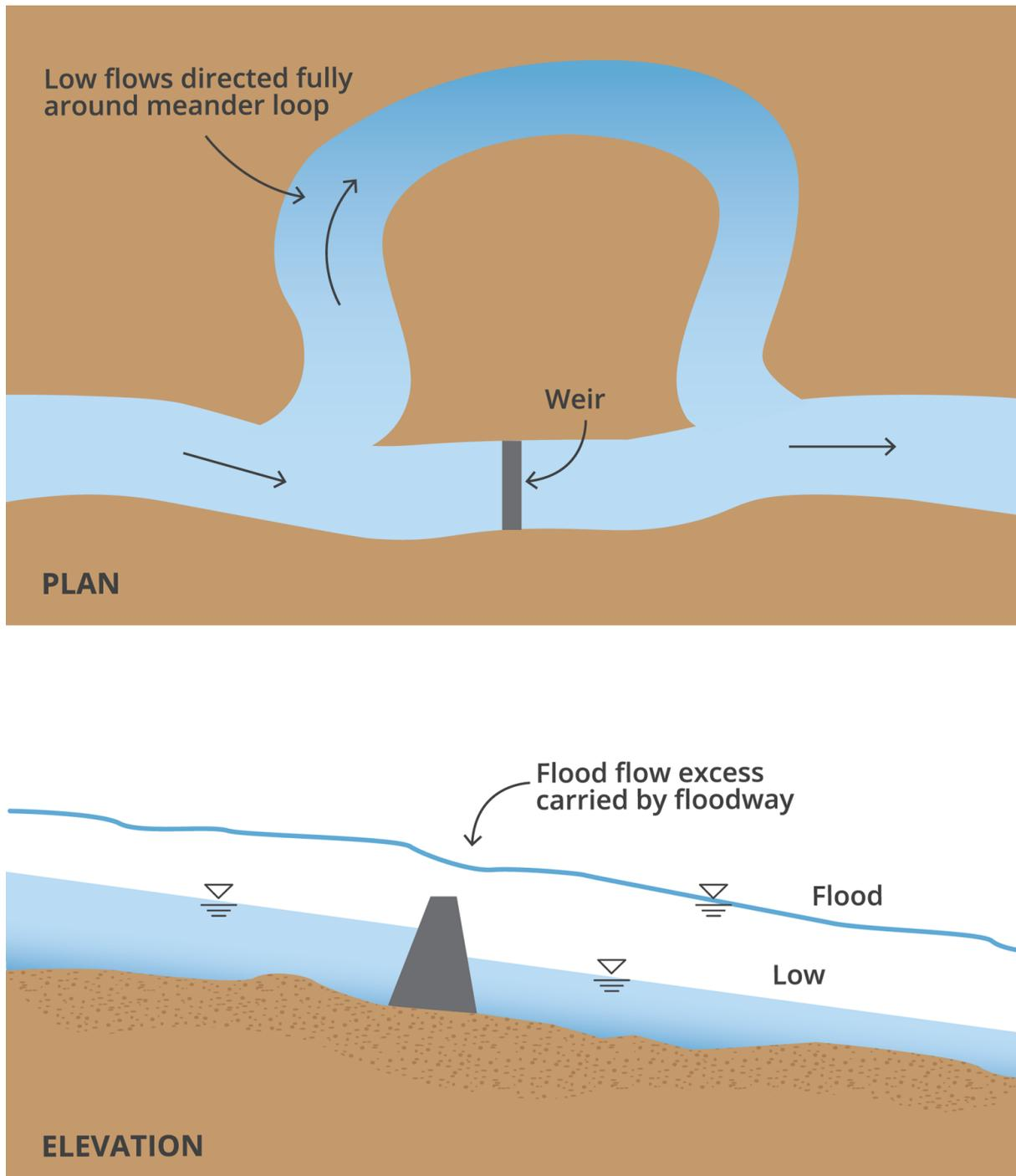
Figure 6.3.1. Schematic of Meander, Floodway, and weir
