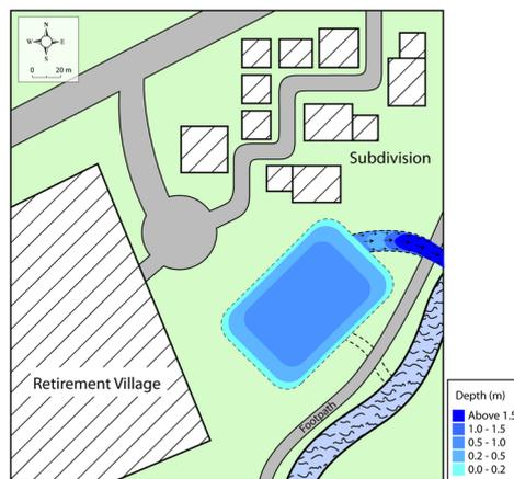
Figure 6.7.20. Basin Overflow Spillway – Flood Depth
