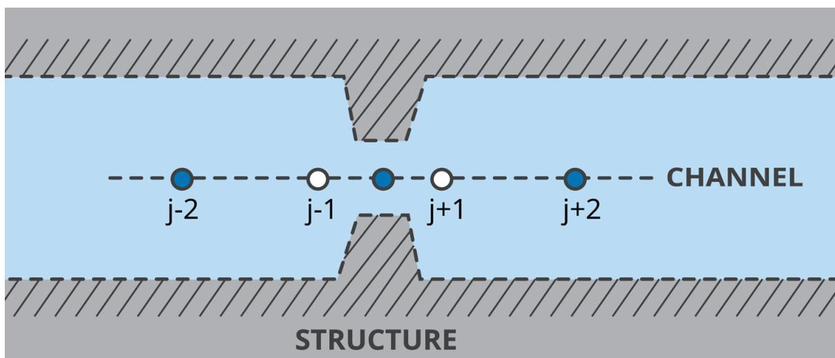
Figure 6.4.5. Schematisation of a Channel and Structure Grid
