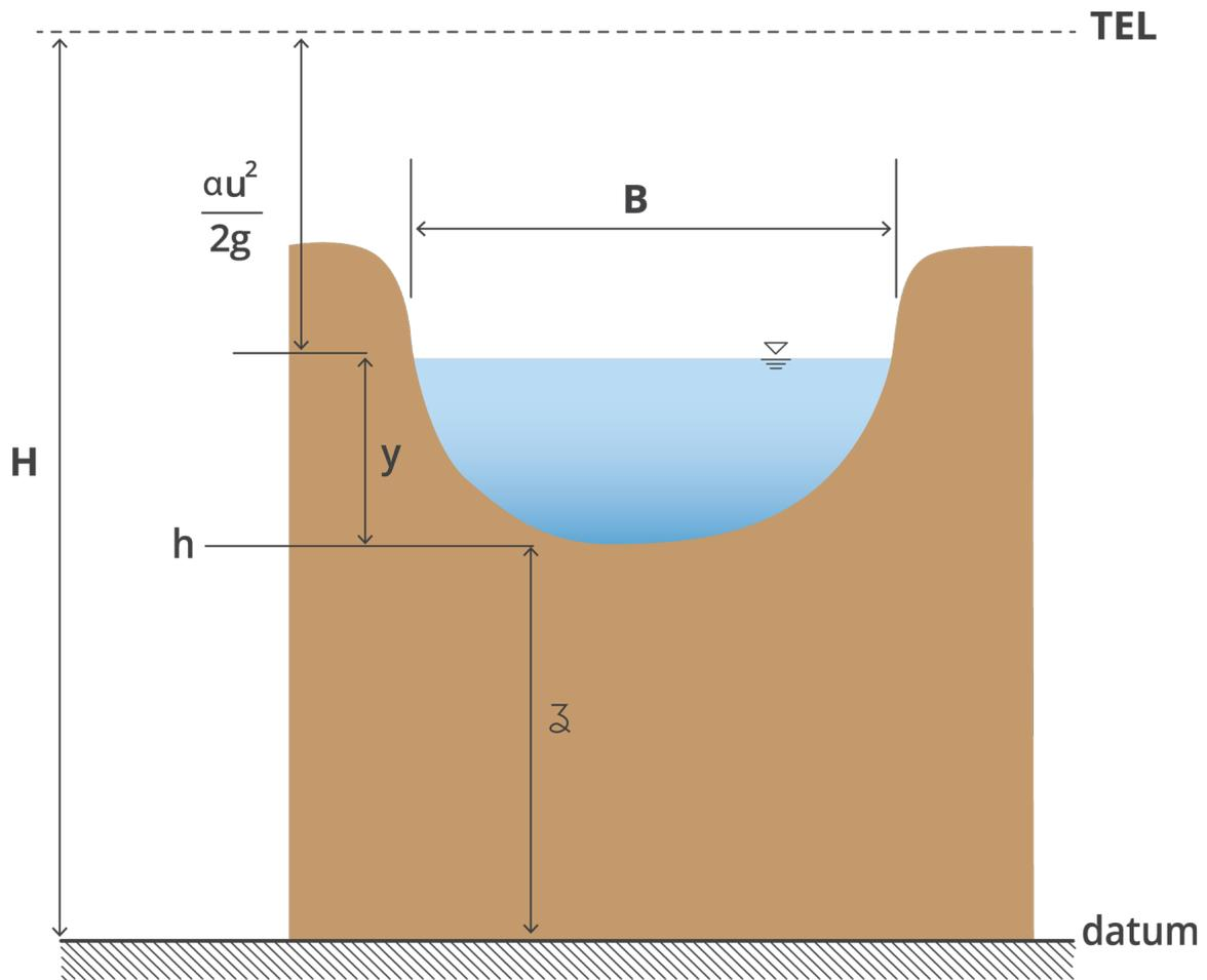
Figure 6.2.4. Parameters characterising flows in open channels
