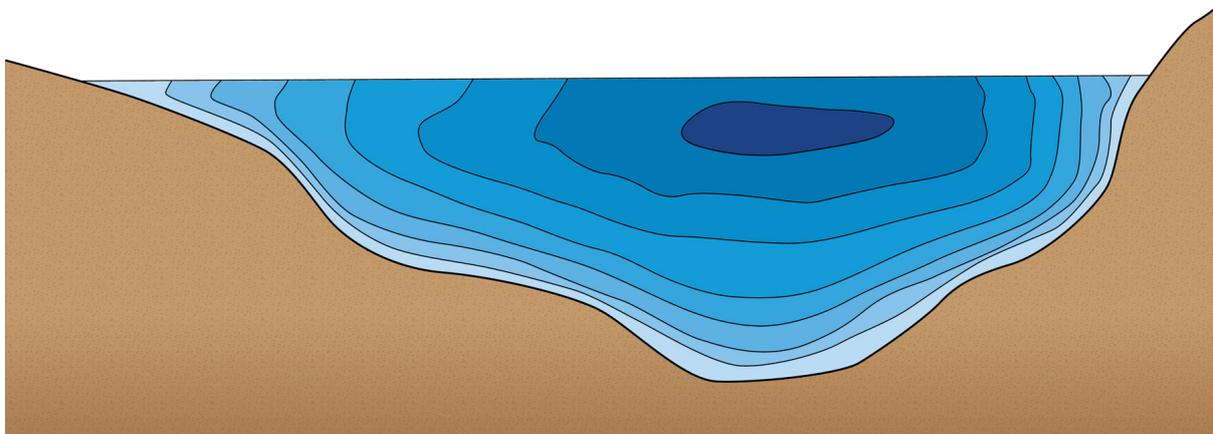
Figure 6.2.7. Typical velocity distribution in a natural channel cross-section
