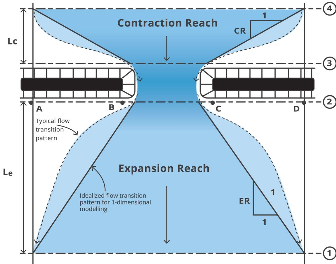
Bridge losses within the expansion reach downstream (sections 1 to 2) can be relatively large. The region is characterised by recirculation zones on either side that are maintained by extracting energy from the mean flow. Energy losses through the contraction (sections 3 to 4) are relatively smaller because the channel length over which the change in cross-section occurs is less and the recirculation zones are smaller.
