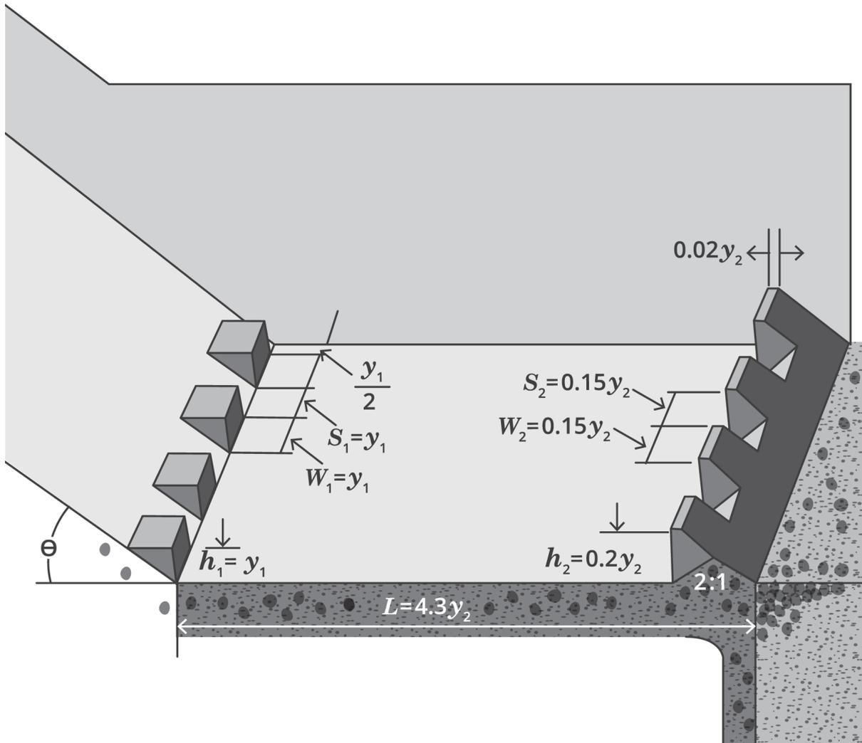
Figure 6.3.5. Schematic of USBR Type 2 Stilling Basin
