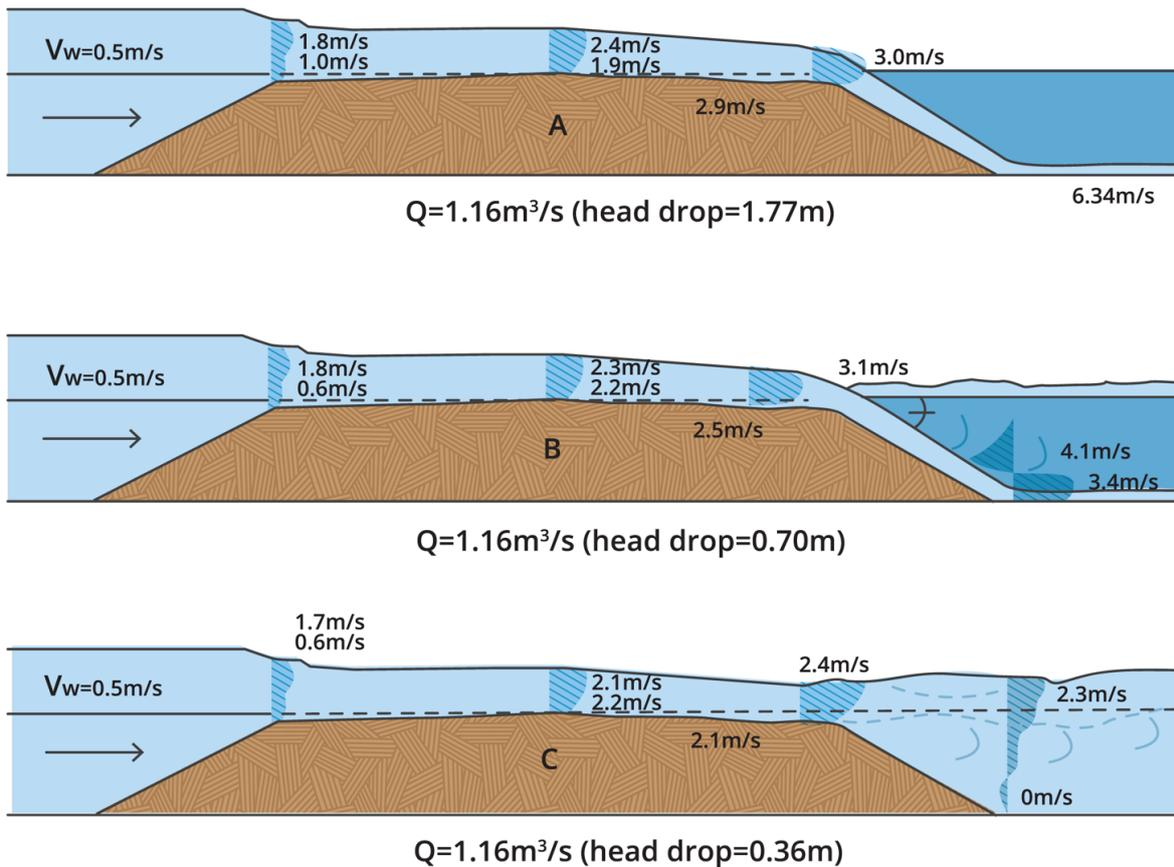
NOTE: The two velocities given at each section represent the maximum and boundary velocities at the section
