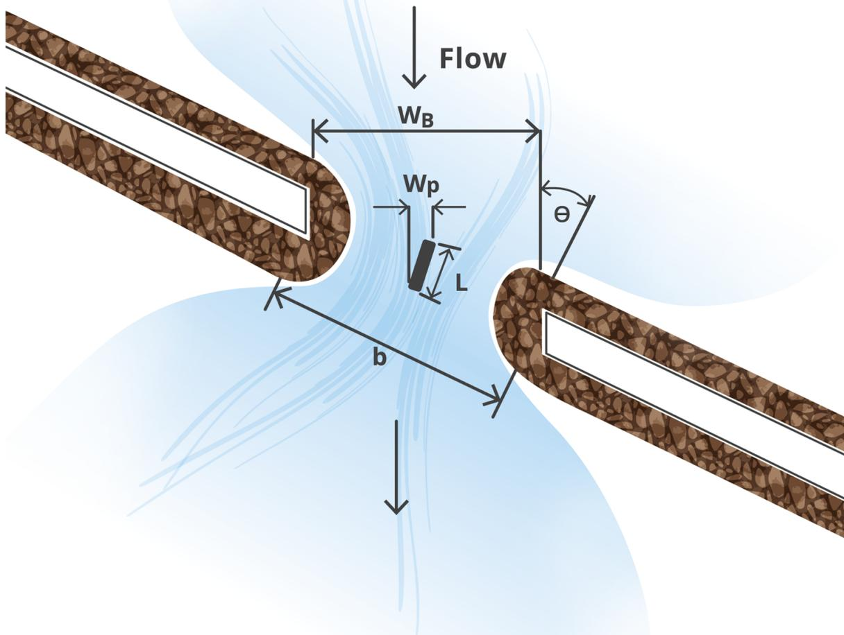
Figure 6.3.15. Schematic of a Skewed Bridge
