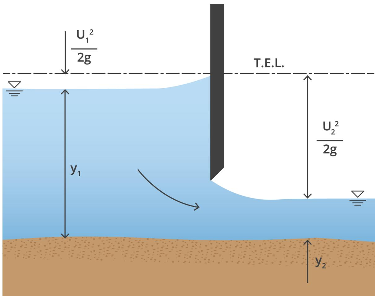
Figure 6.3.3. Schematic for flow under a Sluice Gate
