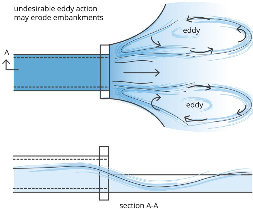
Figure 6.3.11. Schematic of Flow at Unsubmerged Outlet
