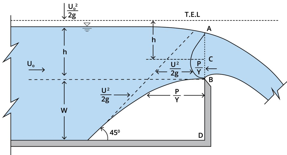
Figure 6.3.26. Schematic of Flow Over Rectangular Sharp-Crested Weir
