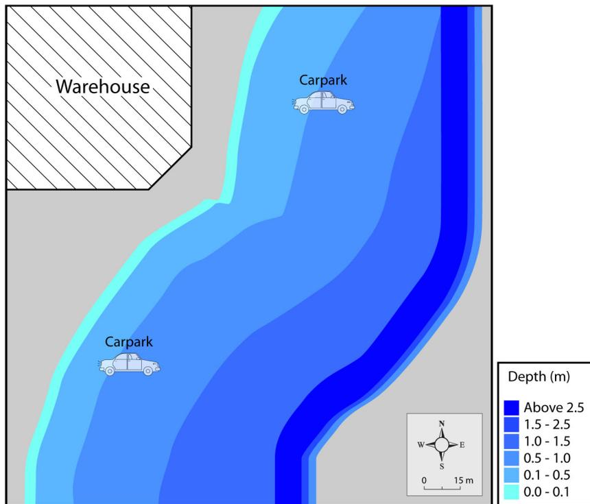
Figure 6.7.13. 1% AEP Flood Depth Map – Existing Site
