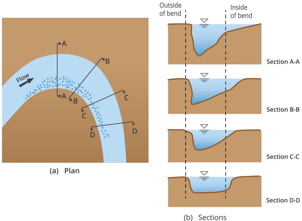
Figure 6.2.5. Variation of cross-sectional properties in natural channel
