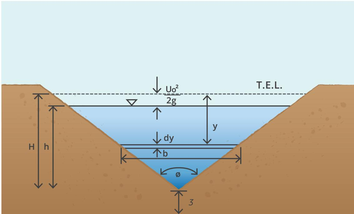
Figure 6.3.27. Schematic of Flow Over V-notch Sharp-Crested Weir
