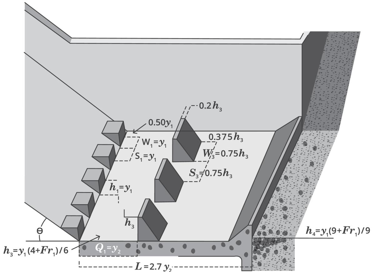
Figure 6.3.6. Schematic of USBR Type 3 Stilling Basin
