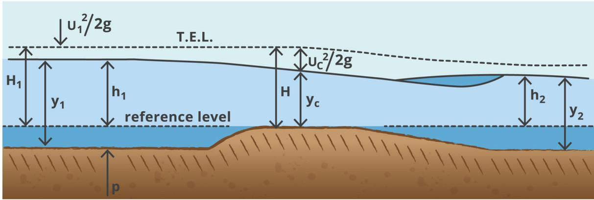
Figure 6.3.30. Flow Profile Through a Long-Throated Flume
