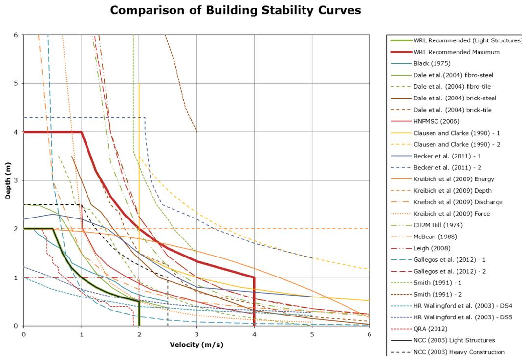
Figure 6.7.7. Comparison of Building Stability Curves
