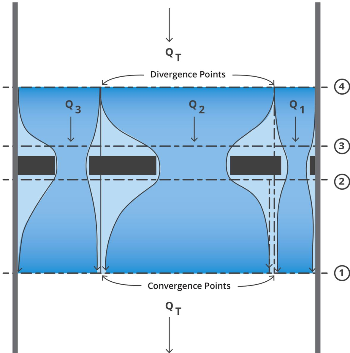
Figure 6.3.17. Schematic of Bridge with Multiple Openings
