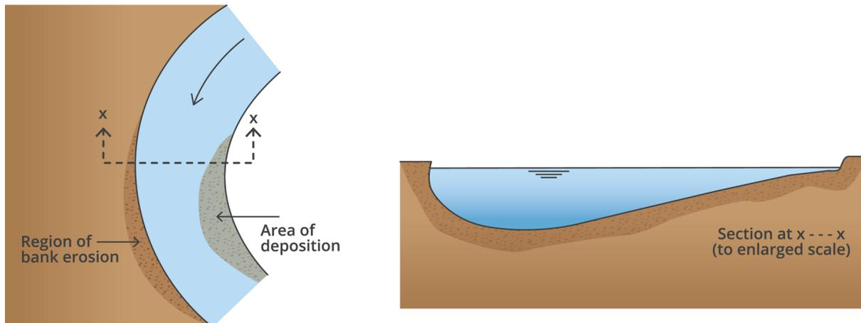
Figure 6.2.3. River bend showing areas of deposition and erosion and characteristic cross-section.
