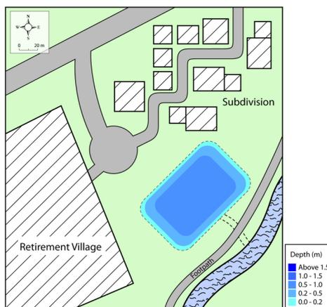
Figure 6.7.18. 1% AEP Flood Depth - Proposed Flood Detention Basin
