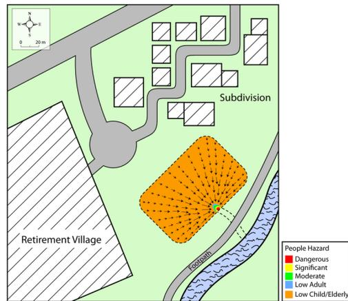
Figure 6.7.19. 1% AEP Provisional Flood Hazard Map - Proposed Flood Detention Basin
