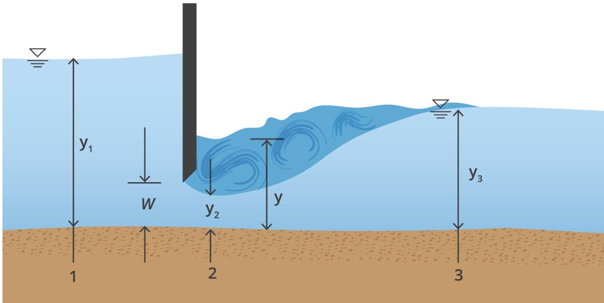
Figure 6.3.4. Schematic of Drowned Vertical Sluice Gate
