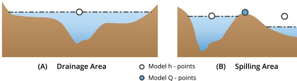
Figure 6.4.6. Different Types of Flood Plain Flow
