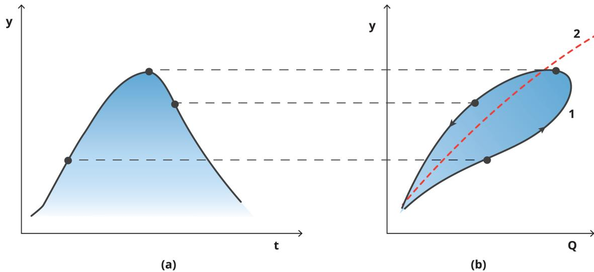
Figure 6.4.2. Storage Effects on the Rating Curve; (a) Flood Hydrograph, (b) Corresponding Rating Curve ([Cunge et al., 1980](#))
