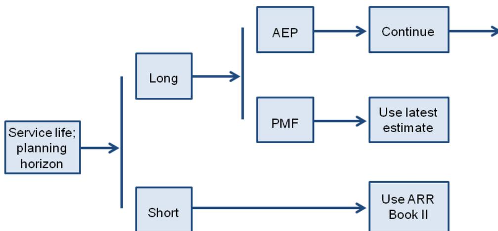
Figure 3a. Decision tree for incorporating climate change in flood design – Part A (AEP = annual exceedance probability; PMF = Probable Maximum Flood)
