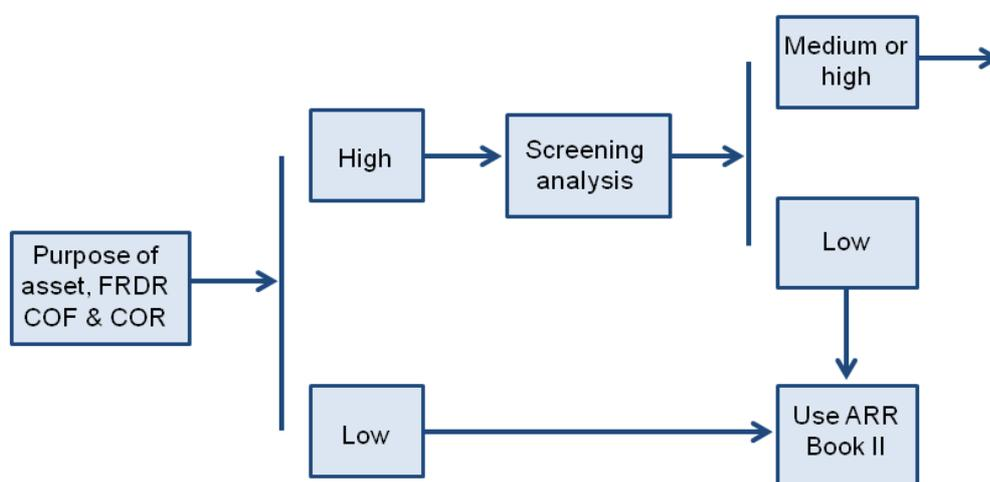
Figure 3b. Decision tree for incorporating climate change in flood design – Part B (FRDR = flood-related design requirements; COF = consequences of failure; COR = cost of retrofits)
