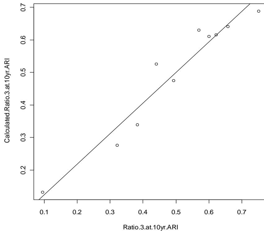
**Figure 98 Fitted values against observed values for cluster 3 Baseflow Volume Ratio regression**
