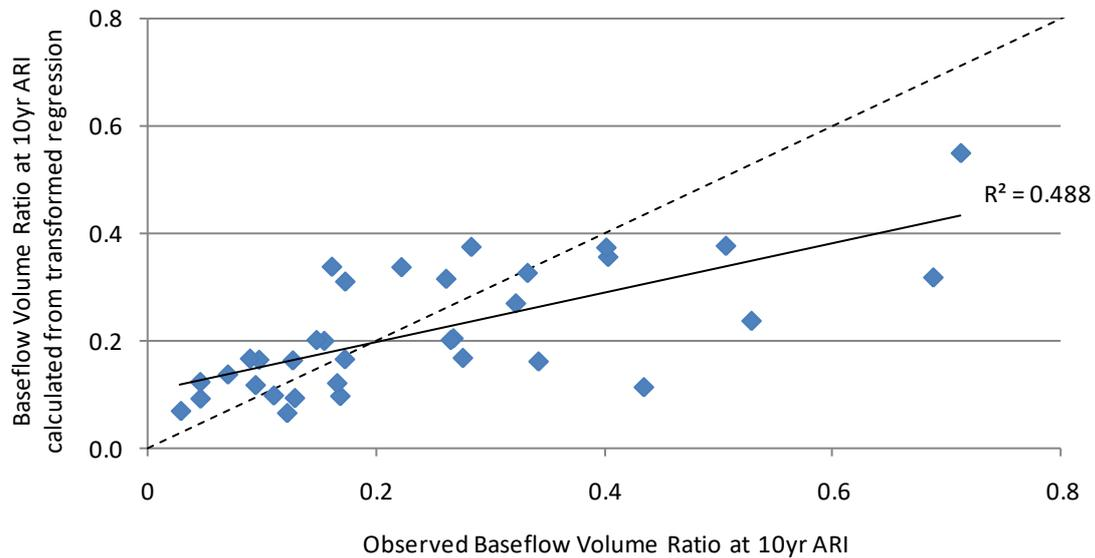
**Figure 35** Observed value of the Baseflow Volume Ratio and the value calculated from final transformed regression for cluster 4. The dotted line shows the one-to-one relationship. The solid line shows the fitted regression.
