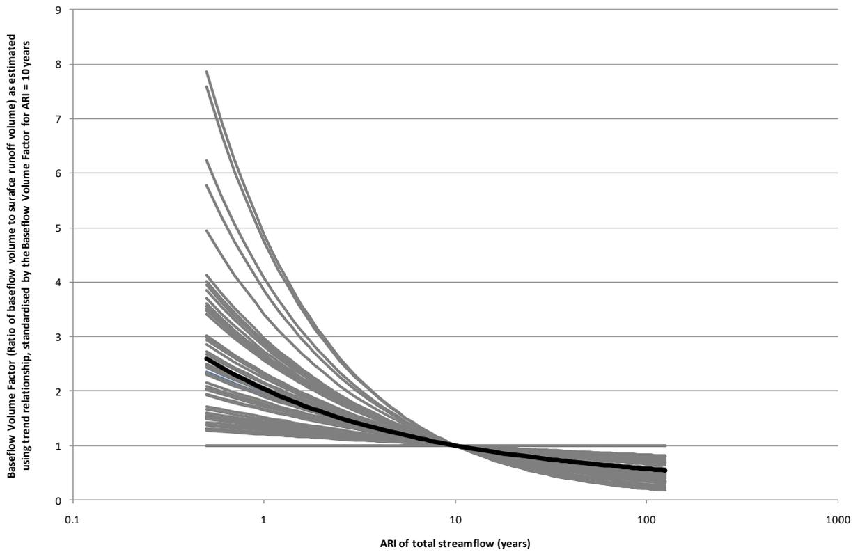
**Figure 56** Summarising the variation in the Baseflow Volume Factor with ARI of the total streamflow for catchments with more than 40 years of streamflow data. The relationship for each catchment has been standardised by the factor value for an event with ARI of 10 years.
