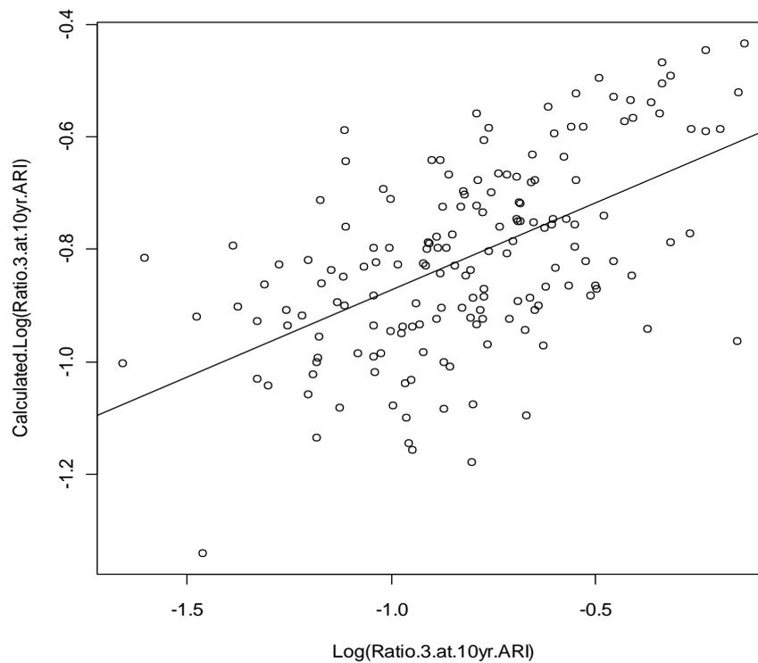
**Figure 88 Fitted values against observed values for cluster 1 Baseflow Volume Ratio regression**
