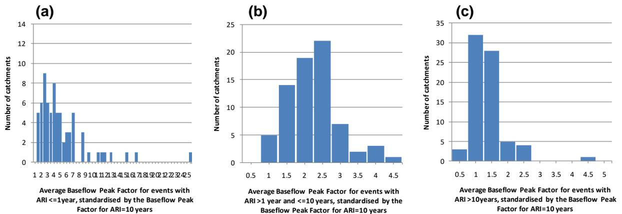
**Figure 53** Frequency histogram of Baseflow Peak Factor for (a)  $ARI \leq 1$ ; (b)  $1 < ARI \leq 10$ ; and (c)  $ARI > 10$
