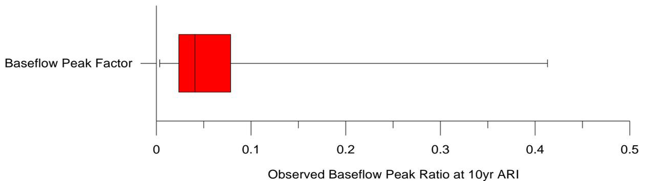
**Figure 27** Box and whisker plot of the observed Baseflow Peak Ratio for cluster 1. The central line in the box represents the median ratio value, the ends of the box reflect the first and third quartiles of the data and the extent of the whiskers shows the range in the data values.
