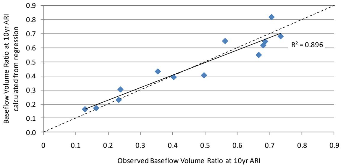
**Figure 33 Observed value of the Baseflow Volume Ratio and the value calculated from final transformed regression for cluster 2. The dotted line shows the one-to-one relationship. The solid line shows the fitted regression.**
