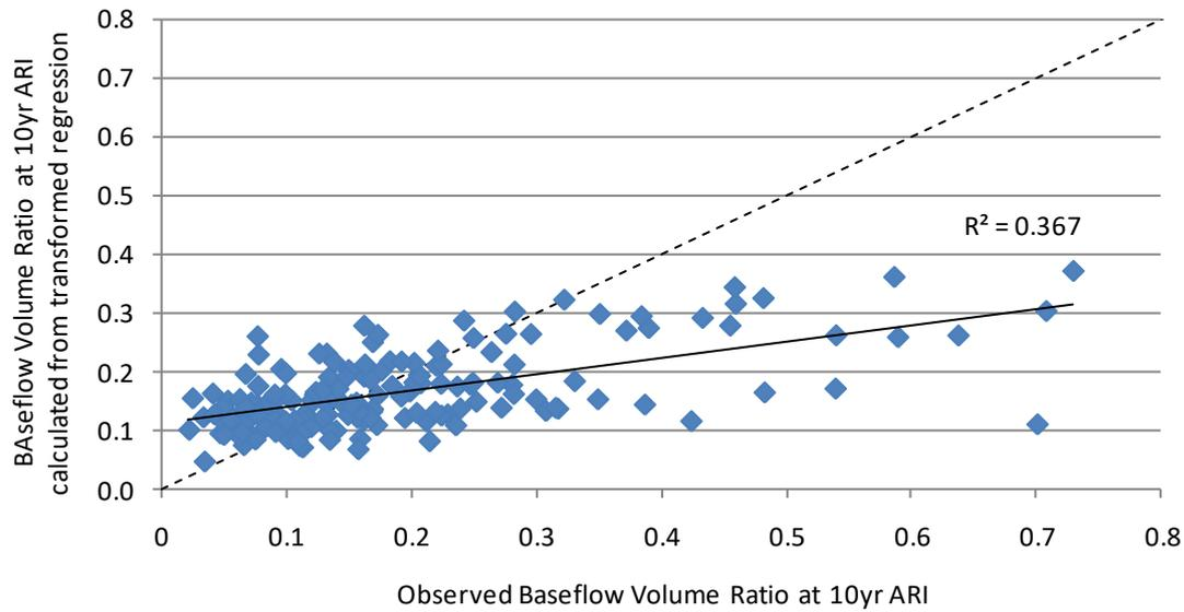
**Figure 32 Observed value of the Baseflow Volume Ratio and the value calculated from final transformed regression for cluster 1. The dotted line shows the one-to-one relationship. The solid line shows the fitted regression.**
