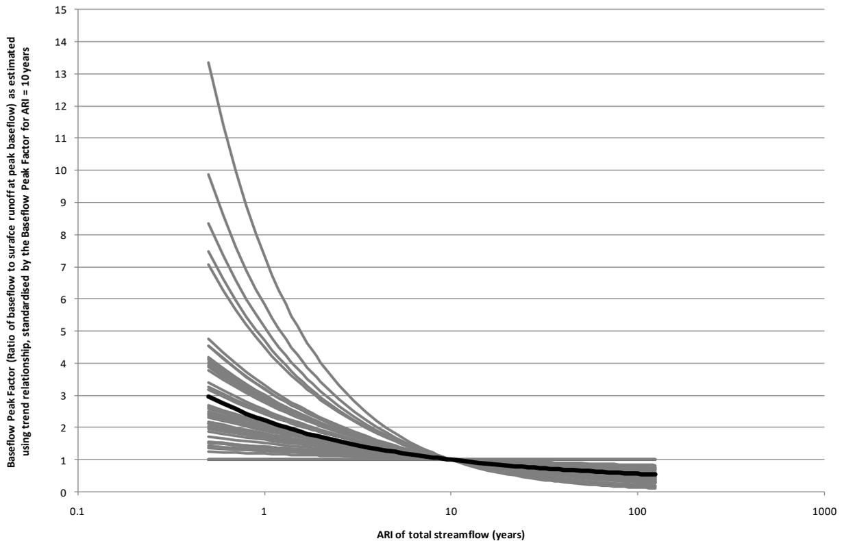
**Figure 52 Summarising the variation in the Baseflow Peak Factor with ARI of the total streamflow for catchments with more than 40 years of streamflow data. The relationship for each catchment has been standardised by the factor value for an ARI of 10 years.**
