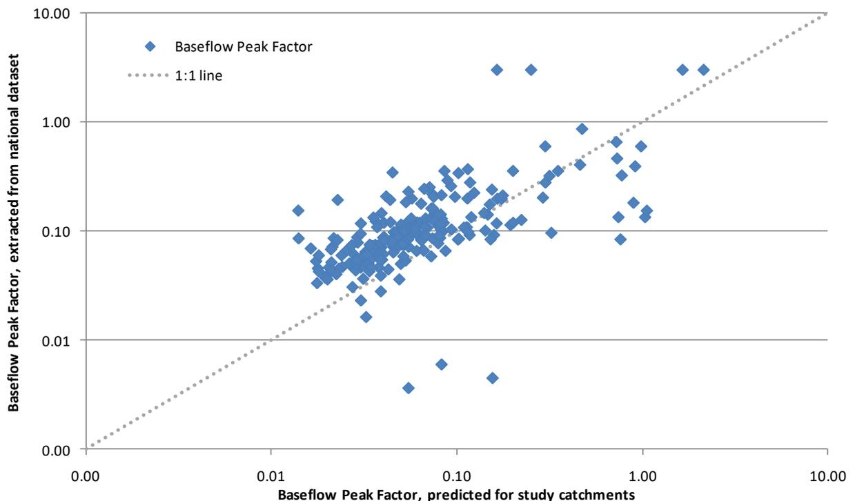
**Figure 60 The Baseflow Peak Factor as predicted for the individual study catchments compared to the Baseflow Peak Factor extracted from the national dataset**
