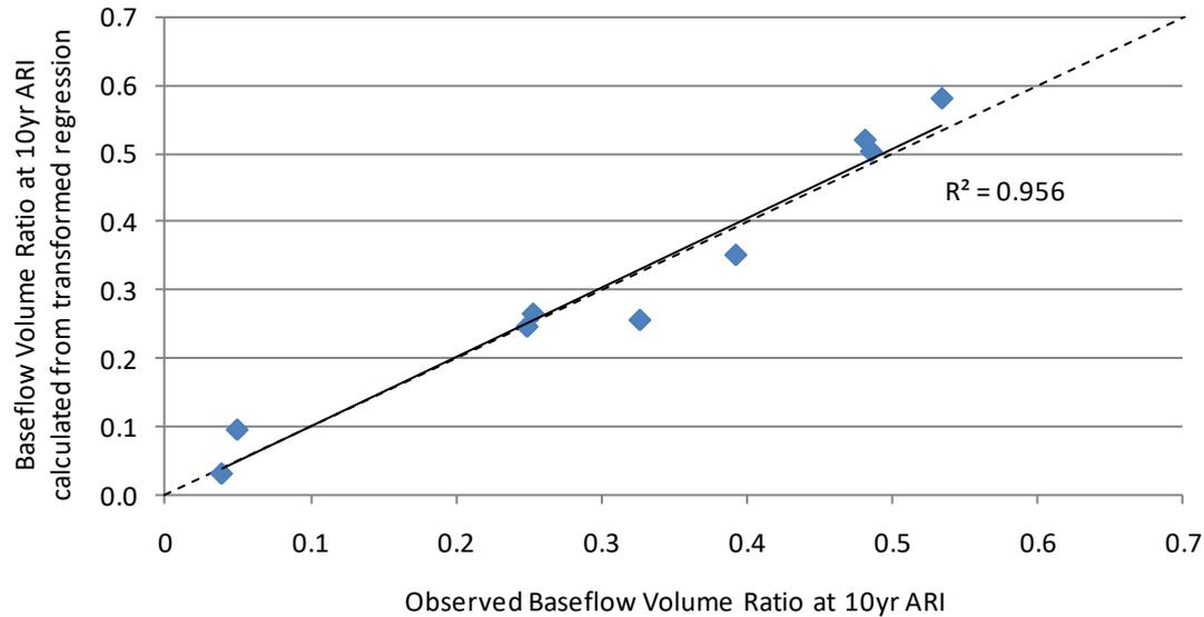
**Figure 36** Observed value of the Baseflow Volume Ratio and the value calculated from final transformed regression for cluster 5. The dotted line shows the one-to-one relationship. The solid line shows the fitted regression.
