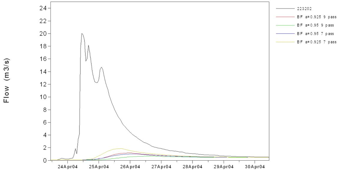
**Figure 8 Example hydrograph showing baseflow separation options for site 223202 in Victoria**
