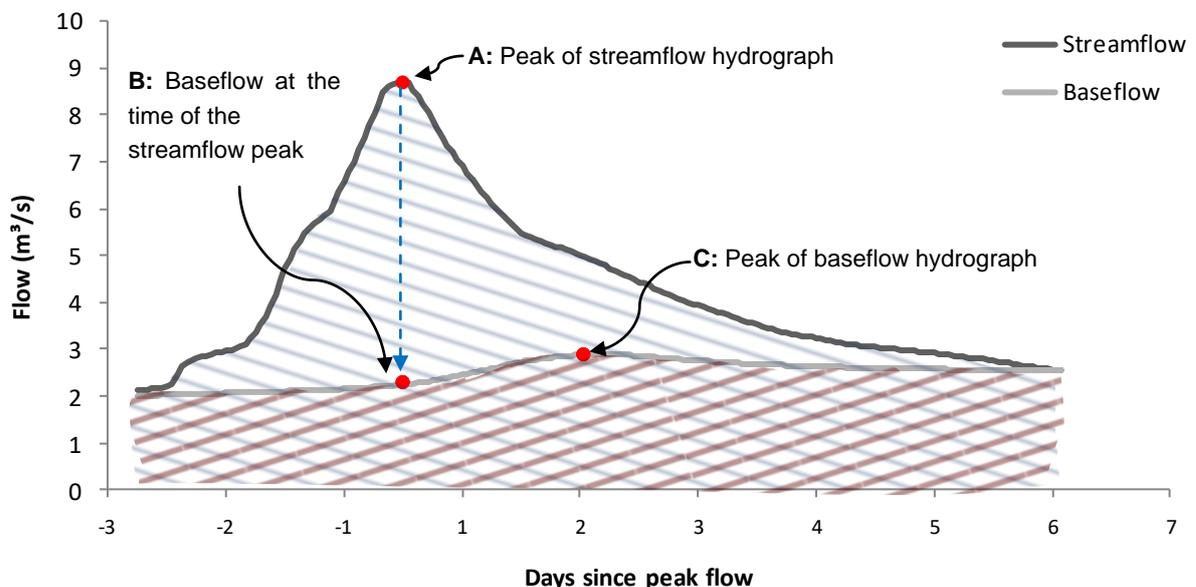
**Figure 14 Flow hydrograph for an event at Victorian site 229214 (Little Yarra River at Yarra Junction) displaying key features**
