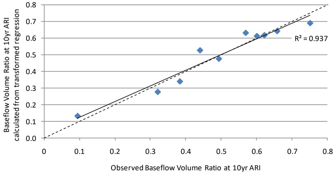
**Figure 34 Observed value of the Baseflow Volume Ratio and the value calculated from final transformed regression for cluster 3. The dotted line shows the one-to-one relationship. The solid line shows the fitted regression.**
