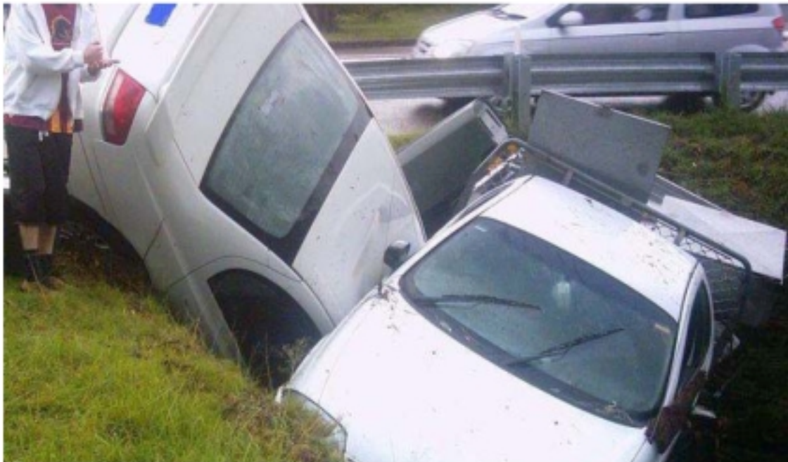
Figure 3.3 – Vehicles Blocking a Culvert Inlet
