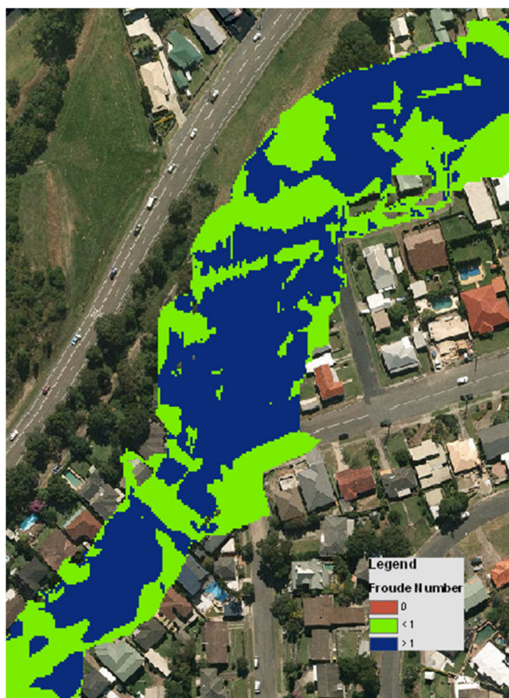
Figure 26: Numerical Model: Froude Number Analysis for the Merewether floodplain without Buildings
