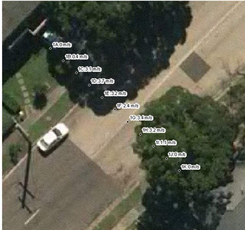
Figure 20: Velocity Measurements: Transect 1
