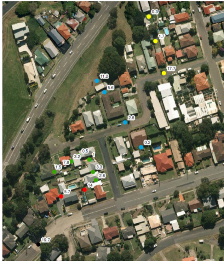
Figure 21: Physical Model: Measured Flows ( \text{m}^3/\text{s} )
