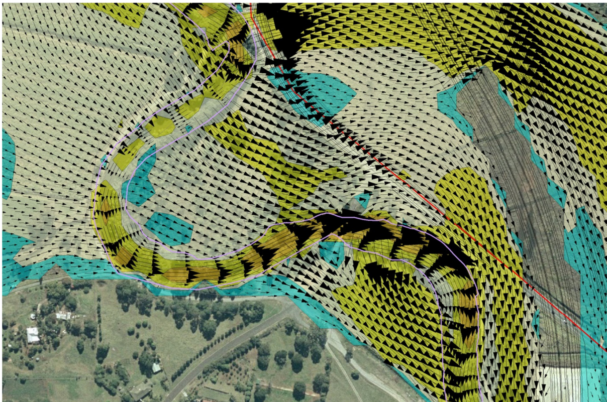
Figure 9-5 Example of 1D/2D Flow Patterns across a Meander using a Horizontal Connection with Momentum Preservation
